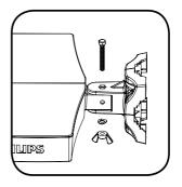
2 Use the screw holes of the wall/mast bracket ③ as a guide to mark position for the wood screws.
